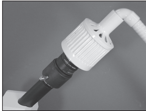
Figure R5.7 | Force Lens Against the Eyepiece
