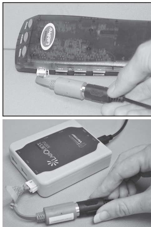
Figure R4.3 | Connecting a Probe to the Interface
