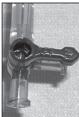
Figure R4.17b | Three-stem valve in position to collect data—flow of gas from syringe is turned OFF.
