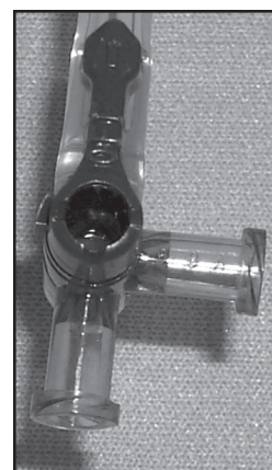
Figure R4.17c | Three-stem valve in position to allow the syringe to remove air bubbles from tubing—flow to sensor is turned OFF.
