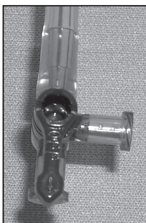
Figure R4.17a | Three-stem valve in OFF position—cuts off the flow of gas from the experimental sources.
